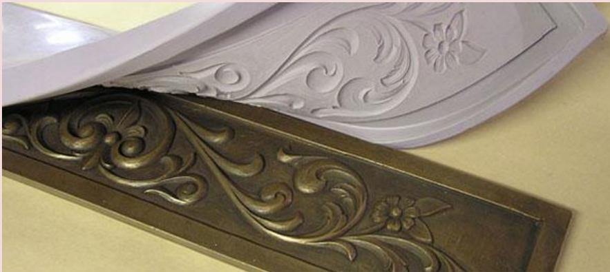
Silicone Moulding Rubbers are used in a variety of industries to produce exact replicas of an original product.
